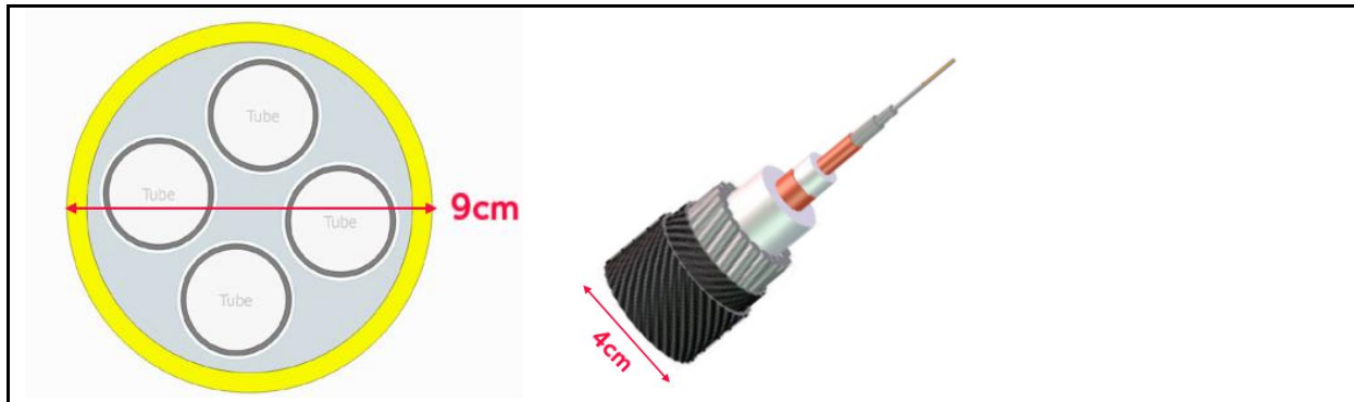
Figure 3-15 Typical structure and cross-section of fluid cable (on the left) and power and signal cable (on the right).
